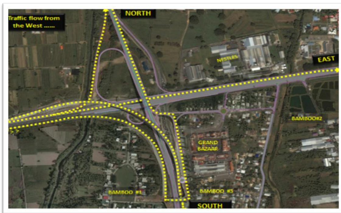
Traffic flow on the Interchange from the West when completed
