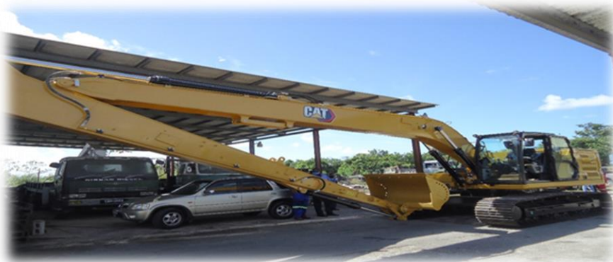
Hydraulic long reach excavator
